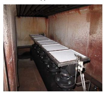
Based on our SB 505 burner module, capacity is added in ½ million Btu/hr increments—increasing capacity simply means adding another module. ALZETA applies its design expertise to select a burner array to match the internal layout of the boiler. You never need to worry about localized hot spots, bypassing, or non-uniform performance.
